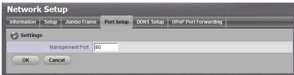
6. Click the **DDNS Setup** tab to enable Dynamic Domain Name Server function, allowing you to connect unit with dynamic IP address.
