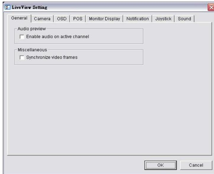
5. Check the **Enable audio on active channel** option to enable audio streaming on active channel. This function synchronizes with right click on camera to enable audio.
