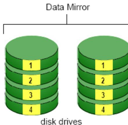
The RAID Volume's data capacity equals the smaller disk drive. For example, a 100 GB disk drive and a 120 GB disk drive have a combined
