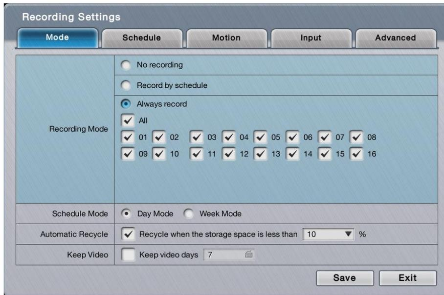
The **Recording Settings** submenu features four tabbed page: **Mode**, **Schedule**, **Motion**, **Input and Advanced**, which are detailed in the following of this section.
