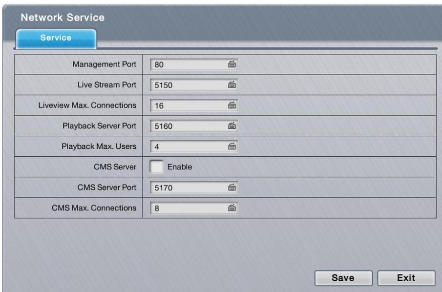
**Network Settings** submenu features one tabbed pages: **Service**, which is detailed in the following of this section.
