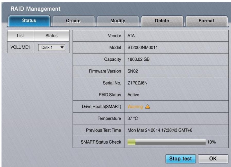
Click the **Stop Test** button to stop the test.
