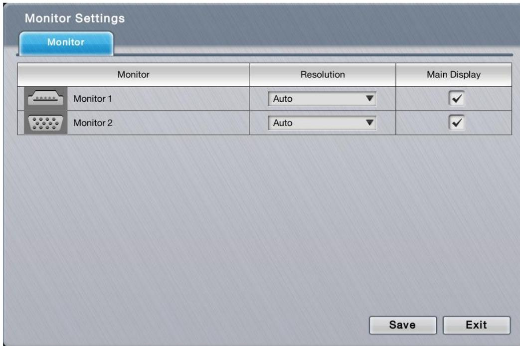
In this page, system allows user to choose both VGA & HDMI as Main Display in the meantime.
