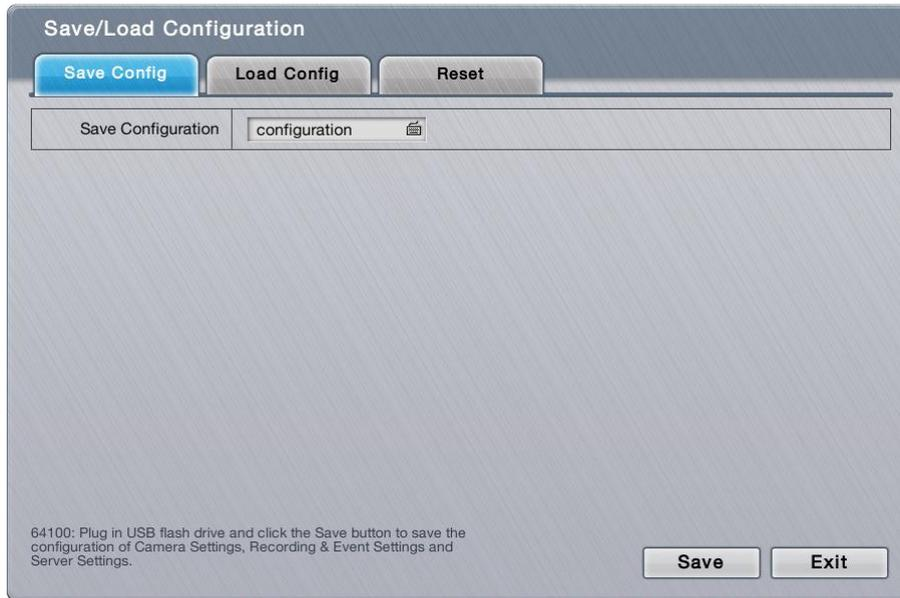
**Save/Load Configuration** submenu features three tabbed pages: **Save Config**, **Load Config** and **Reset**, which are detailed in the following of this section.
