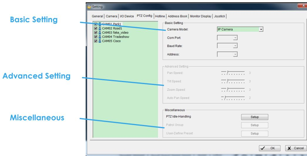
Install PTZ cameras and follow the instructions of the camera manufacturer. A PTZ camera is usually connected to the PC with RS-485/RS-422.
